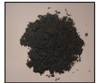
Digital photograph of ultrathin graphene nanoplatelets (in bulk quantity)
